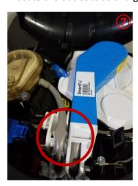
• Close the blue latch securely, close the cooler top and continue to prime if necessary.
